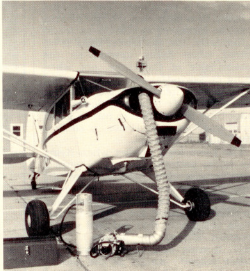
Fast engine preheaters, like the Flame Engineering model shown, can help you be on your wintry way in just minutes while helping extend the life of your engine.
